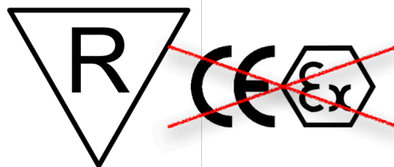
Fig.8. A post-repair device with explicit conformity marking (R in a triangle) indicates that a significant change has been made.
