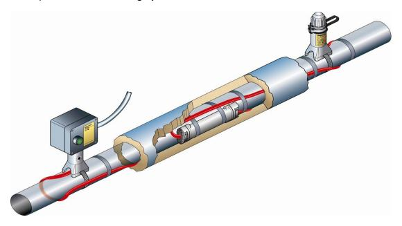
For design, installation and maintenance, the application guide EN 60079-30-2 may be used, this guide is written in conjunction with the product standard EN 60079-30-1, according to which trace heating systems for use in potentially explosive atmospheres are usually assessed and certified.
