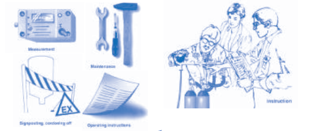
Figure 4.1. Examples of organisational explosion protection measures (12)
